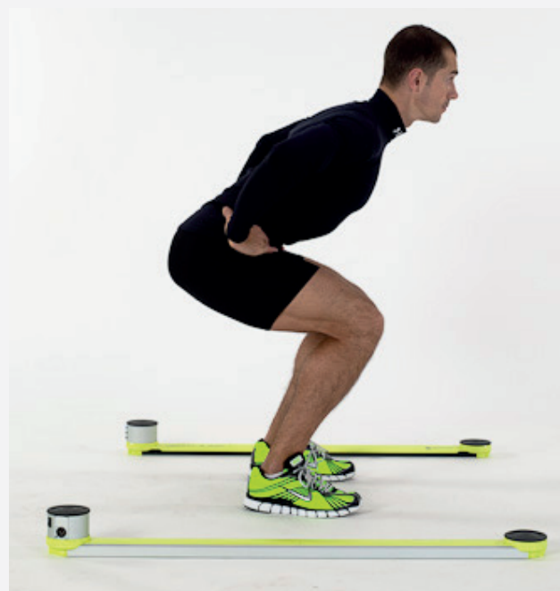
Picture 2. Assessment of squat jump height using Optojump Next system.
