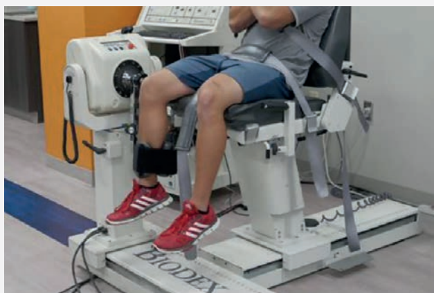
Picture 3. Assessment of muscular performance using isometric instrumented system.
